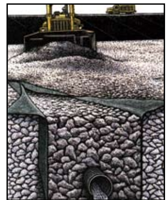
Geotex® woven monofilament geotextiles are very resistant to biological clogging, making them ideal for landfill leachate collection systems.
